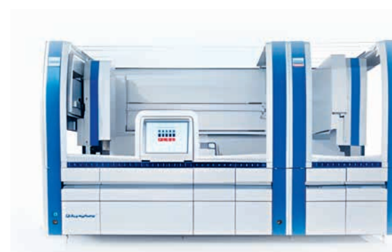
SLIKA 6.4. Qiagen QIASymphony® SP Instrument za automatsku DNA izolaciju (preuzeto i prilagođeno s https://www.qiagen.com/ja-us/products/diagnostics-and-clinical-research/sample-processing/qiasymphony-dsp-dna-kits-us , pristup 3.10.2023.).
