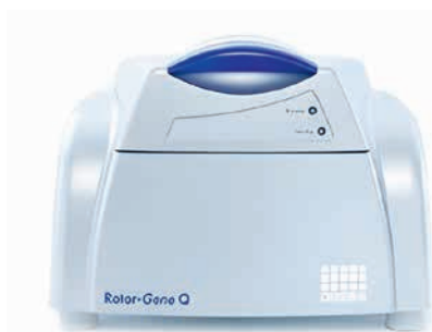
SLIKA 6.17. Rotor Gene Q rtPCR system (preuzeto i prilagođeno s https://www.qiagen.com/ja-us/us/products/discovery-and-translational-research/epigenetics/dna-methylation/methylation-specific-pcr/rotor-gene-q , pristup 28.7.2024.).
